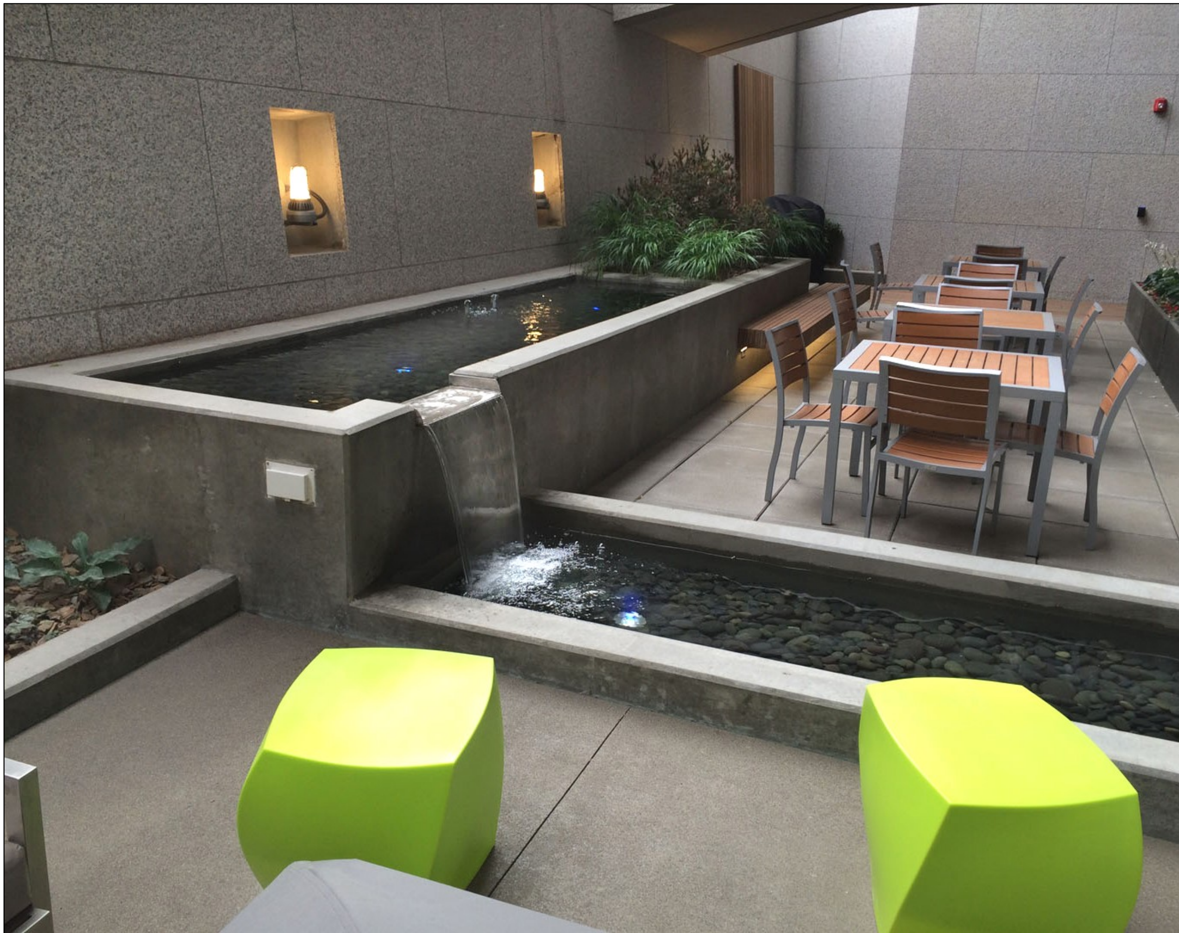
Sheet falls mute street noise, but in this small walled reverberating area must be kept small enough to not inhibit conversation. Existing wall alcoves were re-purposed for ambient lighting. (North courtyard)
